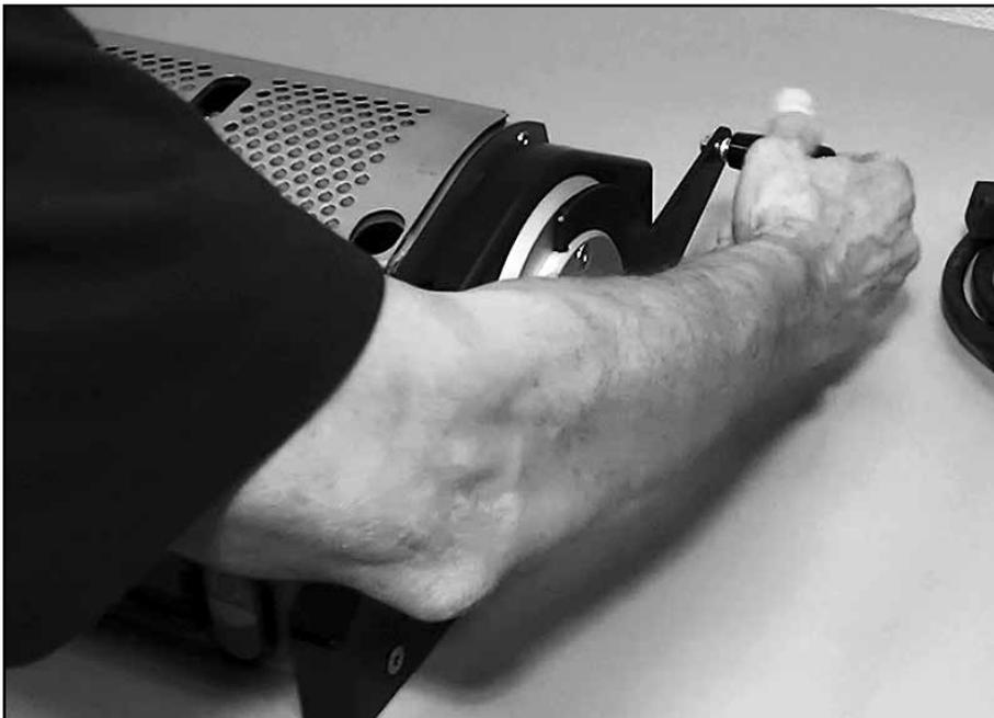
Rotate actuating lever to its operating position.
