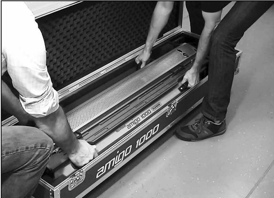
Open transport case and lift machine from case. **Caution!** Two persons required to lift and place machine. Position machine on even surface with platens up and level. Do NOT apply power until belt is cut and clamped in preparation for splicing. Ensure power inlet, controls, and cutter crank are accessible.
