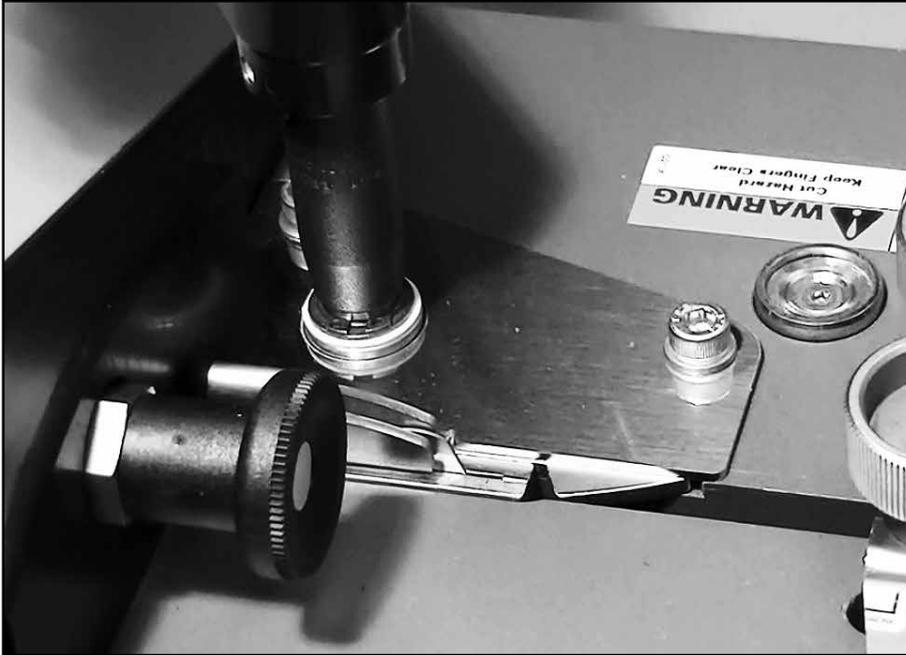
Continue cranking until blade arrives in its stowed position and cutter position latch is activated.
