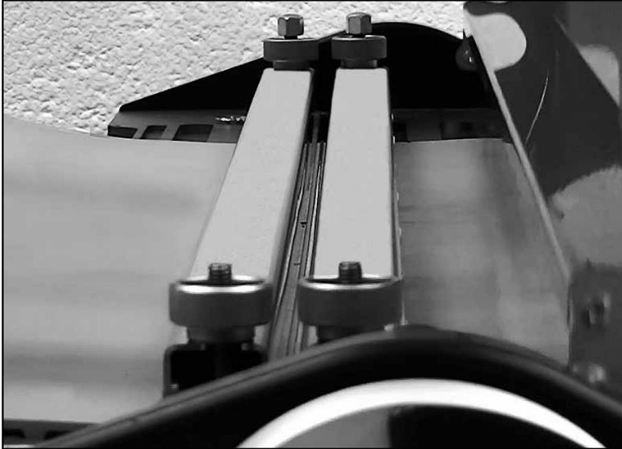
After light signal indicates conclusion of splice process, remove guard.
