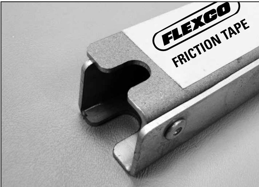
For tension-driven flat belt or positive drive belts with segmented drive features, a preferred practice is to use Flexco Friction tape (Item No. 08604) installed on clamp bars. Friction tape assists in fixing the belt position during the cutting and splicing operations. A damp cloth can be used to clean the friction tape surface.
