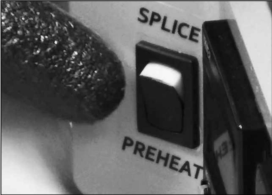
Place heating mode switch to PREHEAT position.
