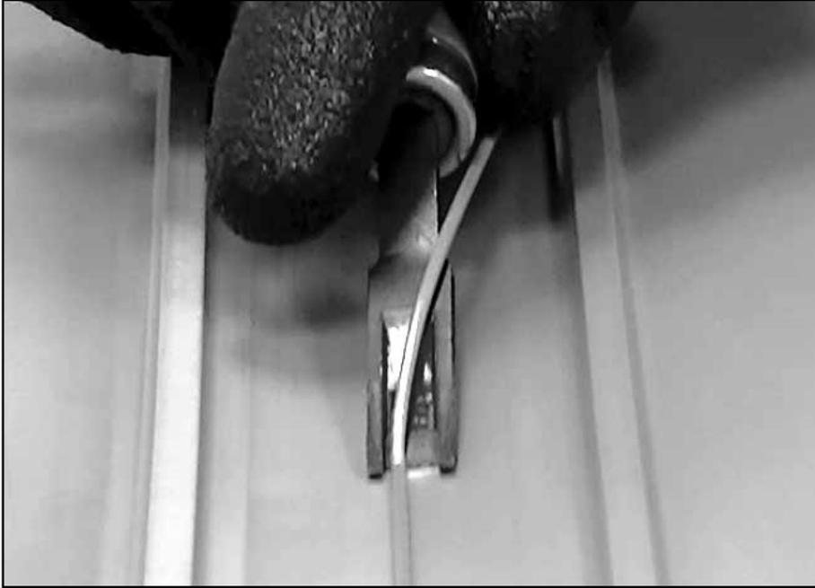
Remove underside weld bead with skiving tool.
