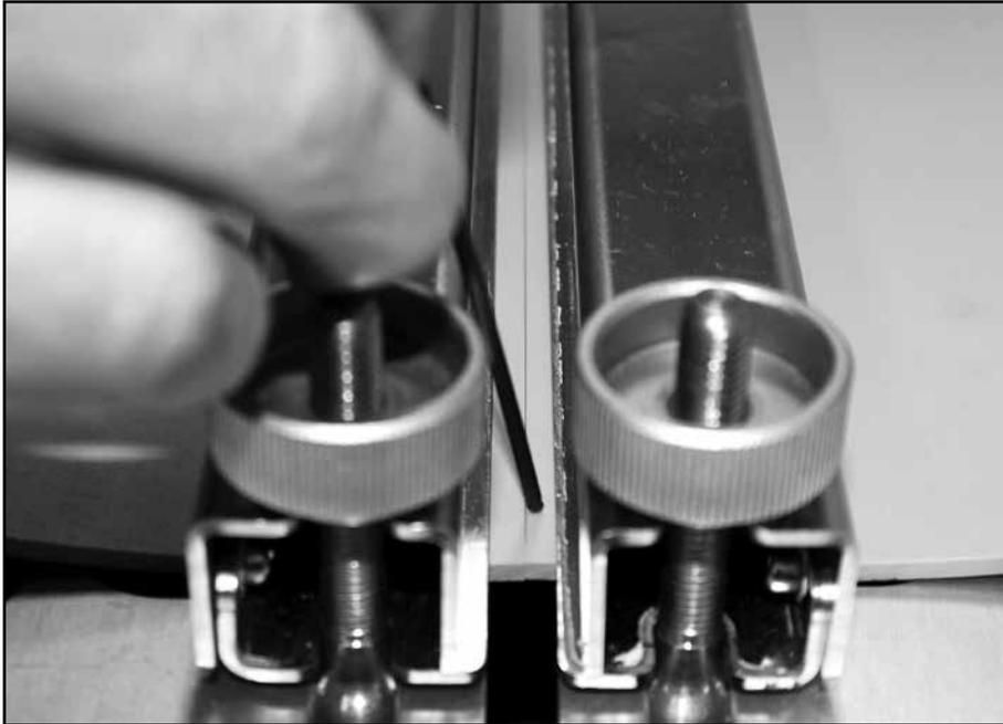
Using 2 mm ball driver provided, or an alternate “probe,” determine by feel if prepared belt ends are uniformly aligned “vertically.” No “step” should be felt when moving probe across cut length. If a step is recognized, attempt alignment of belt surfaces via tightening (or loosening) clamp thumb nuts.
