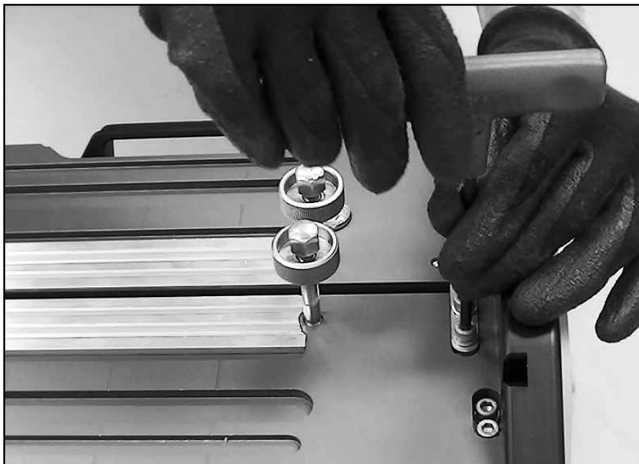
On platen stop plate, loosen two socket head cap screws using a 5 mm hex driver. Repeat for platen stop plate on opposite end of platens.
