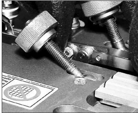
7. Compress emitter spring tensioner to allow emitter mounting hole to be engaged with copper emitter block mounting stud.
