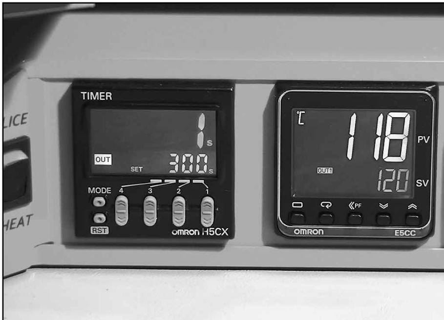
Allow preheat period to expire. A sound tone will be heard at conclusion of preheat cycle. Allow machine and belt to cool to preset "splice start" temperature.
