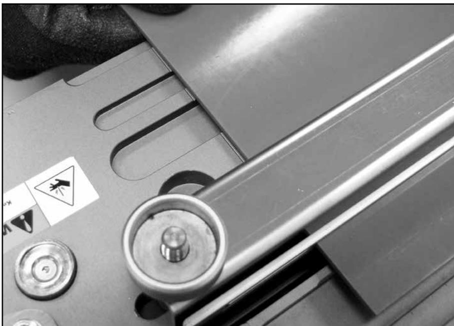
Ensure belt is positioned “square” to machine by either engagement of positive drive feature, or by using a square or alignment marks. **Note!** Belt widths less than 760 mm (30”) should be centered in machine for splicing.
