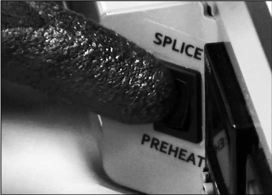
During this cooling period, set heating mode rocker switch to SPLICE position.
