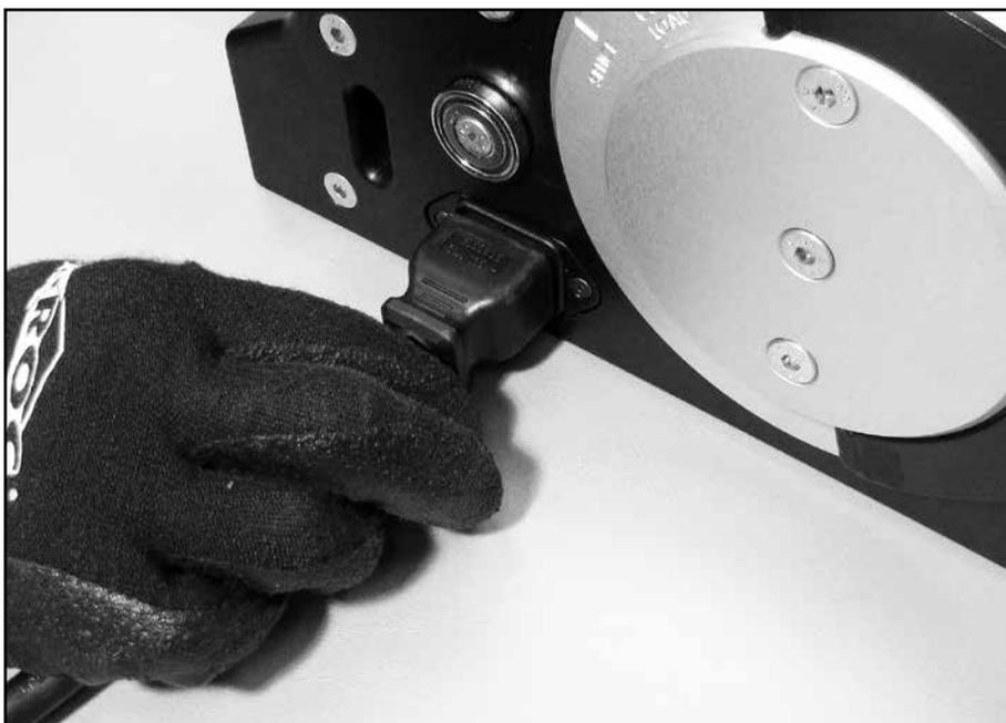
Select proper power cable and plug into machine power inlet.
