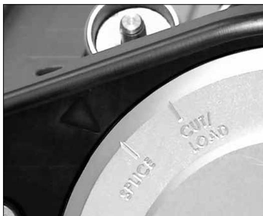
1. Rotate actuator lever to SPLICE position.
