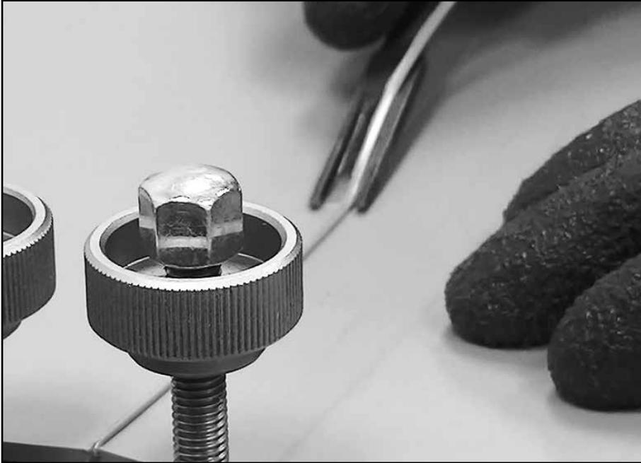
Remove weld bead from top side of belt with skiving tool. This is best accomplished while belt remains on machine with edge positioned against the vertical clamp studs.
