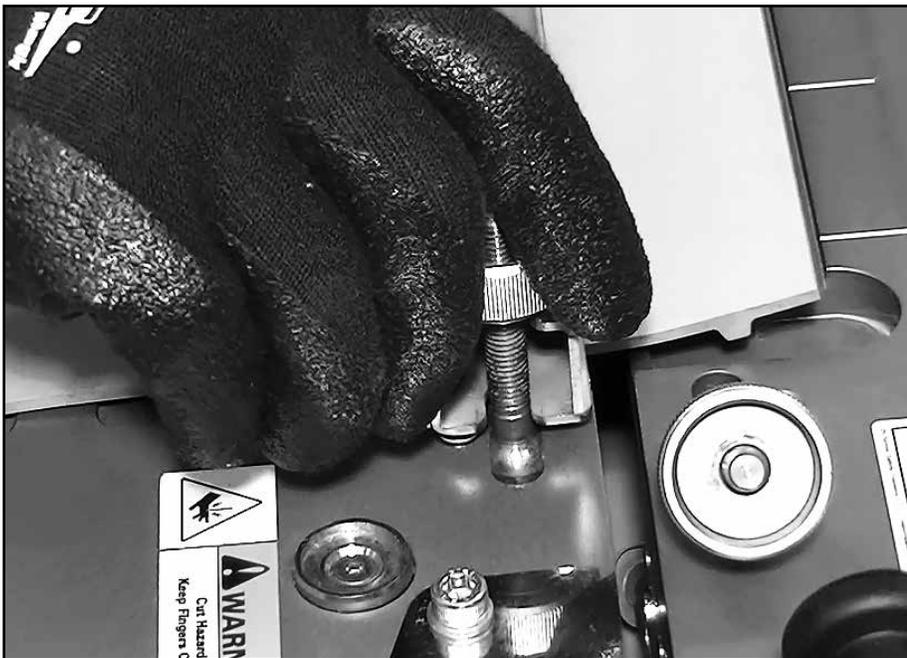
Install one clamp bar tightly over installed belt and template.
