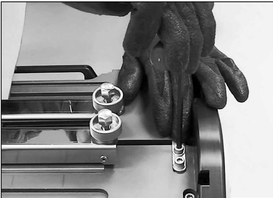
Tighten two socket head cap screws using 5 mm hex driver. Repeat for platen stop plate on opposite end of platens.
