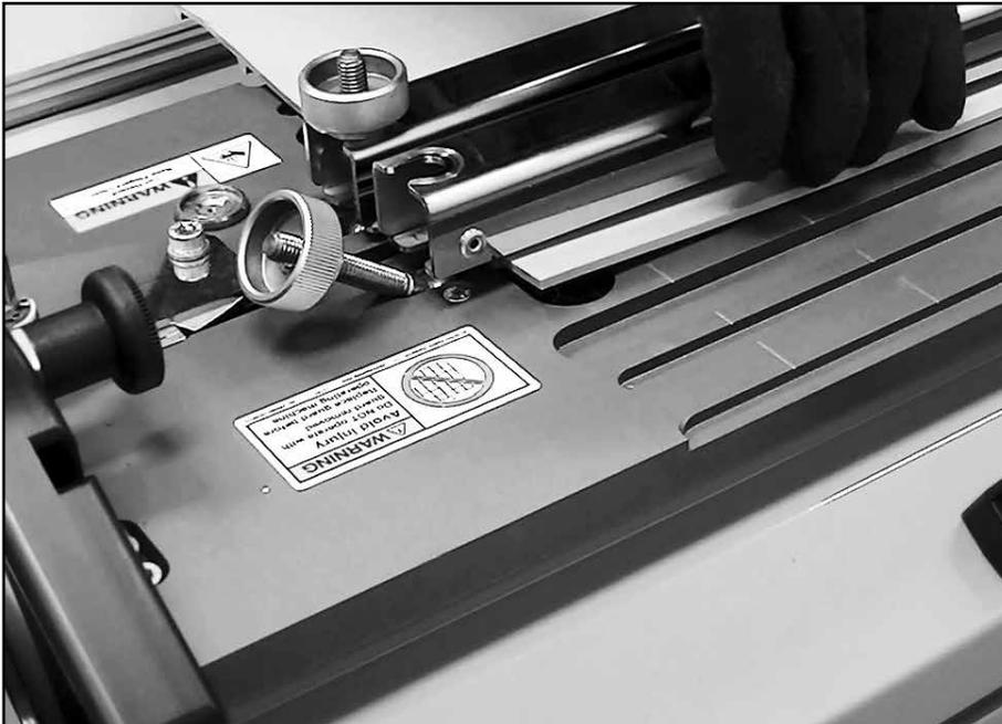
Relax clamp thumb nuts and remove clamp bars. Move prepared belt end clear of machine.
