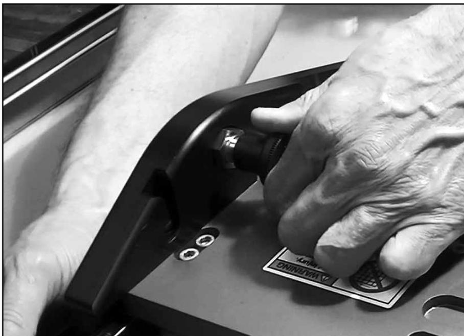
Lock in place with locking pin.
