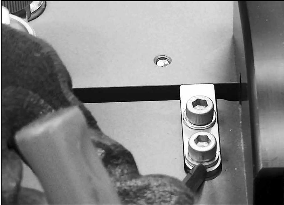
Move platen stop plate to contact fixed platen face. Repeat for platen stop plate on opposite end of platens – move to contact blade holder.
