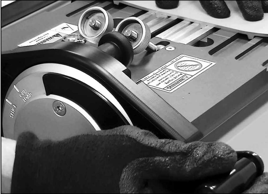
Position belt with drive bars engaged in both templates. Rotate actuating lever loosely between “Cut/Load” and “Splice” positions.
