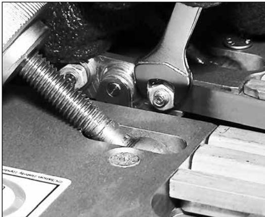
8. **DO NOT RELEASE SPRING COMPRESSION.** Premature release of compression spring load may cause damage to emitter mounting hole. Ensure emitter is seated in copper emitter block recess. Install Belleville washer over mounting stud with large washer contact area side against emitter strip. Install retention nut and tighten to fully compress Belleville washer. Spring compression may now be released.
