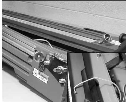
4. Swing control end platen side out of front plate retention grooves. Place platen near machine.
