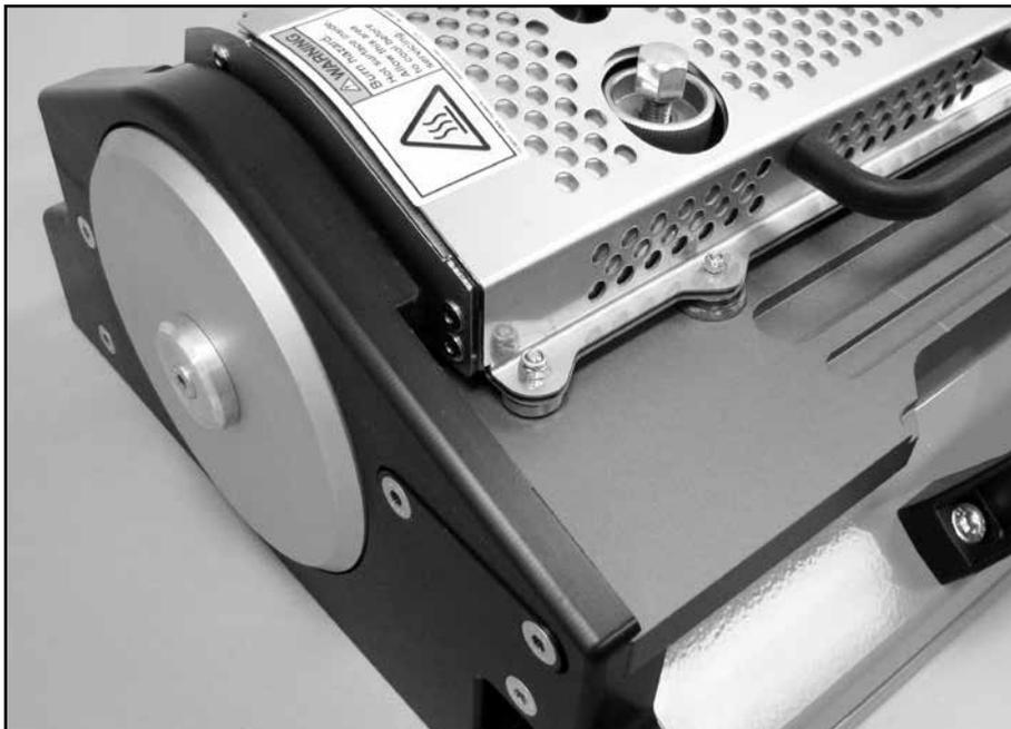
Install guard and ensure magnetic engagements are secure and seated.
