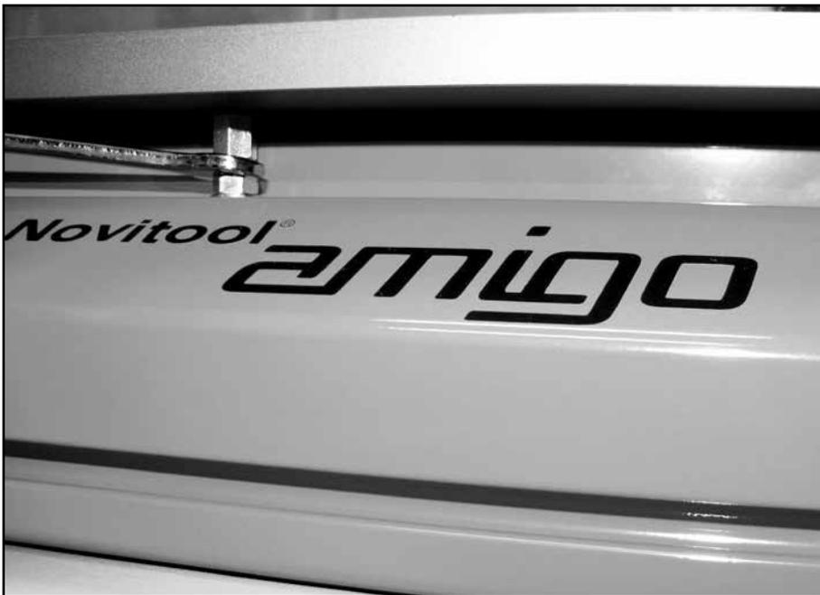
If belt surface cannot be aligned by thumb nut tension, fixed platen can be adjusted using two jacking screws. Ensure jacking screws are locked into position, using associated jam nuts once belt surface alignment is achieved.
