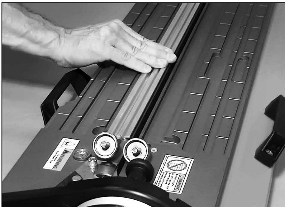
Ensure only one template is installed.
