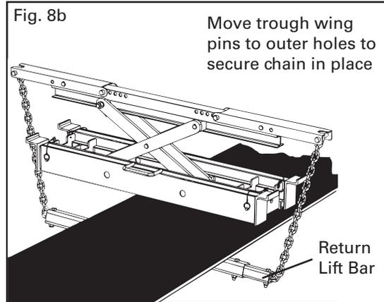
**STEP 10. Lift the Belt.** Turn the Adjusting Nut counter-clockwise until the belt is at the desired height. (Use the correct size socket and tool—not included.) Remove the ratchet or power tool prior to starting work.
