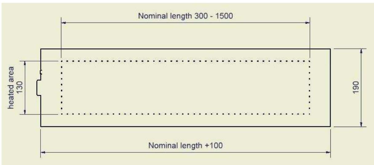
*(Splice plate dimensions and the heated area)*
