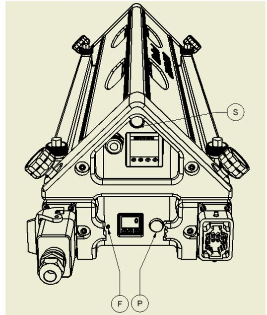
Release pressure by pushing button "P". Hold the button until all pressure is released to zero. The actual pressure is displayed in the controller.
